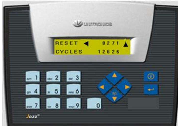
A compactor should be serviced about every 15,000 cycles. The oil should be changed, and the photo eyes cleaned, and the alignment checked. The first line of this display shows the number of cycles since the last oil change. This counter is reset by touching the left arrow key. The second line displays the lifetime number of cycles. The maximum count is 9,999,999. At this point the counter will automatically reset to zero.
