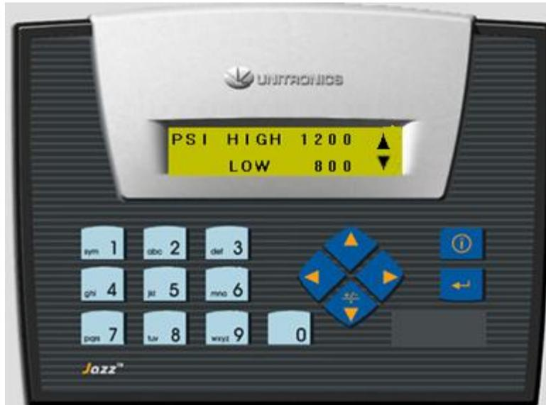
The maximum allowable pressure setting is 1600 PSI for high pressure and 1200 for low pressure. The *Up Arrow* key will take the operator back to Serial Number. The *Down Arrow* Key will allow him to adjust timer setpoints.
