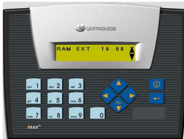
Ram Ext is the time in 1/100 of a second that the ram travels forward at the start of compaction. If the time is set too short, the compaction will not be maximized. If the time is set too long, the compactor will reach a mechanical stop and a high pressure COMPACTOR FULL alarm will occur.
