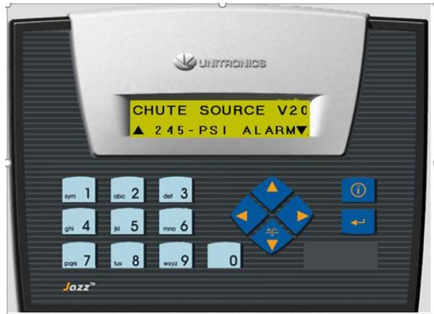
On power up the unit displays the Model number of the unit – V20. It shows the peak pressure of the ram’s last move. The *Up Arrow* key will move the operator to Manual Control, while the *Down Arrow* will take the operator to Alarms. If there is an alarm present, the word ALARM will appear next to the Down Arrow.
