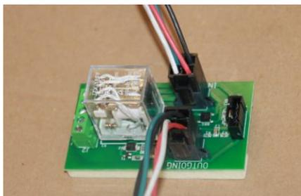
The circuit board is keyed so the cables can not be inserted incorrectly. The board has a plug for the (INCOMING) previous floor and the (OUTGOING) next floor. The cables must not be reversed. The cable length is marked on each cable. The cable connecting the first floor panel with the basement has a threaded locking ring (squeeze fitting). This fitting is required because of the extra wall thickness of the polycarbonate control panel.
