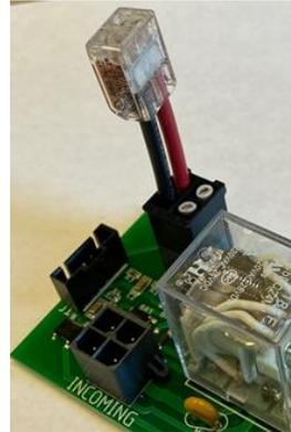
A terminating jumper must be installed on the last floor. This jumper is normally installed by the factory. If an optional heat detector is purchased, it replaces this jumper.
