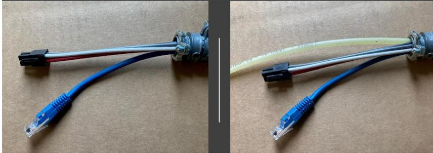
A single MC Cable provides the floor to floor connection. It does not matter whether the system is a BI Sort, TRI Sort or ADA air. The cable includes a 14 gauge, 4 conductor power cable and an ethernet communications cable. For an air operated system, the air supply tubing is also included.
