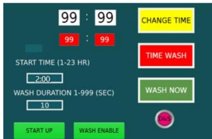
The washdown system allows control from the basement to locations along the chute, designed to wash and disinfect the chute. The control is built into the master control panel, so a separate box does not need to be wired or installed. The wash solenoids connect directly to the floor panels so a MC Cable connection to the basement is not required.
